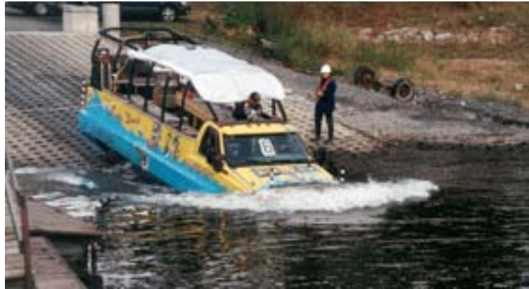
Photo 9. Vehicle launched at 8 km/h, visor submerged by approximately 25 mm
