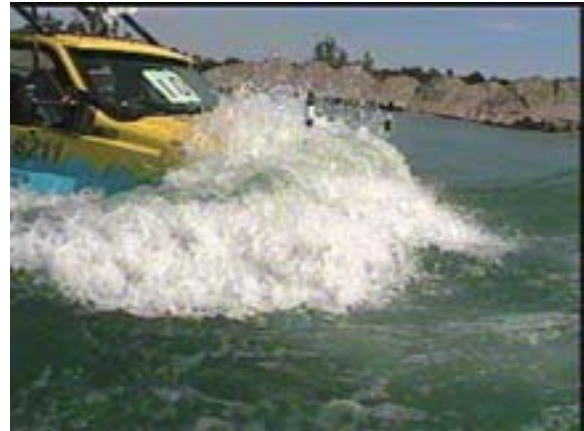
Photo 8. Vehicle speed of 9.75 km/h in disturbed water
