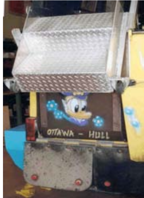
Photo 13. After boarding ramp in retracted position
