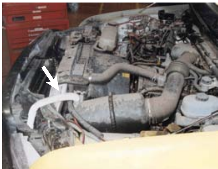
Photo 3. Discharge hose from the forward engine compartment
